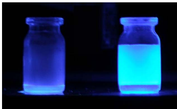
Figure 1. Comparison of appearance of non-fluorescent and fluorescent microspheres exposed under UV light: Without POPOP (left) and with POPOP (right). [Color figure can be viewed in the online issue, which is available at wileyonlinelibrary.com .]
